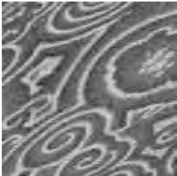
Photoemission electron microscope (PEEM) imaging. Dark regions are predominantly oxygen covered, bright regions are mainly CO covered.
